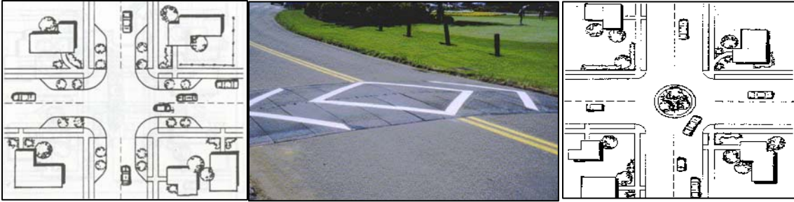
Traffic Calming Devices: “Curb bump-outs (left), speed humps (center), and traffic circles (right) are more effective than stop signs in slowing traffic on residential streets.”
